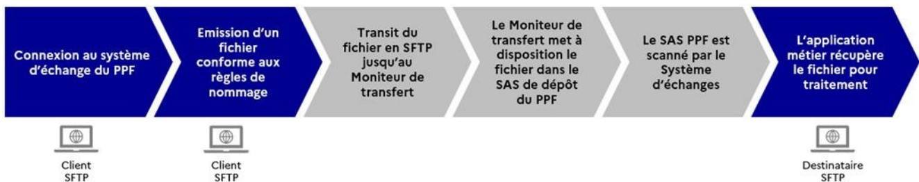
Figure 5 - Flowchart of an incoming data stream via SFTP
