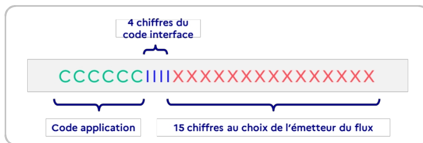
Figure 15 – Recommendation for the composition of a message identifier
