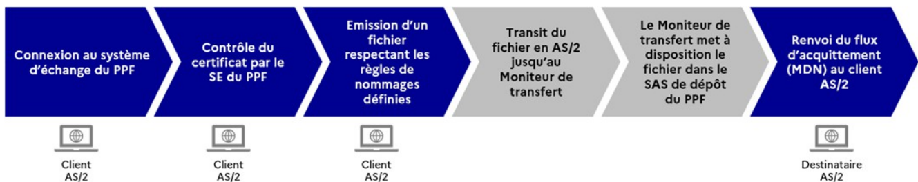
Figure 7 - Flowchart of an incoming stream via the AS/2 protocol
