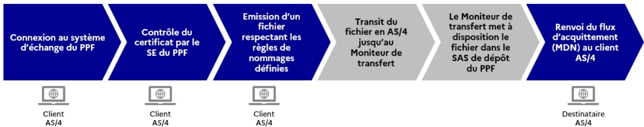
Figure 9 - Flow diagram of an incoming flow via the AS/4 protocol
