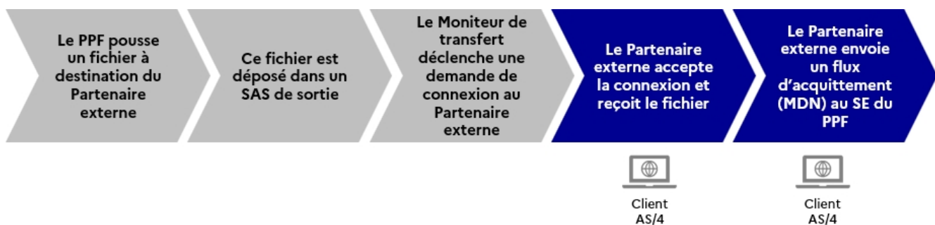
Figure 10 - Flow diagram of an outgoing flow via the AS/4 protocol
